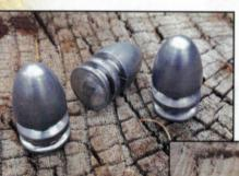
When I was happy with the bullet moulds, one hundred bullets were cast for testing. The Minié' bullets were swaged up to .546 and then lubed with a 50/50 mixture of beeswax and
