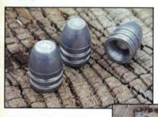
The compression bullet mould cast a .546 bullet at 435 grains in pure lead. While it would work if loaded naked in the bore like a
