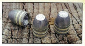
The compression bullets were divided into two groups, sized and unsized. The unsized .546 bullets received a quick dip of the base into melted lube, being careful to not get lube into the compression grooves. Those would be shot naked in the bore like the Minié' bullets.
