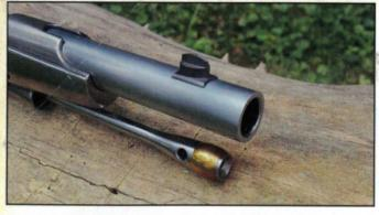
The Minié' bullet mould included for testing cast a 350 grain hollow based bullet that measured .543 as cast in pure lead. But, the diameter really needs to be .547 or .546 for best accuracy. So, a simple hammer swage die was made to "bump" the bullets up to .547. The plug for the bump die was made to match the hollow base, both to ensure it was not damaged, and to uniform the skirt while swaging.
