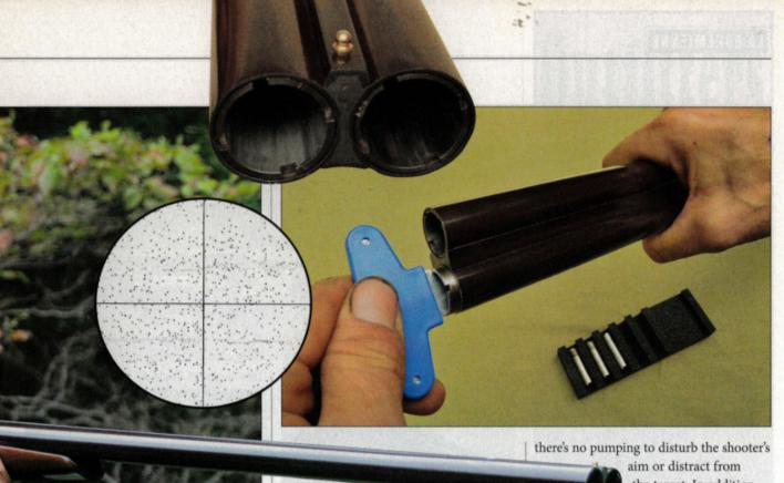
The Pedersoli comes with five screw-in choke tubes and a T-wrench to install them. The author tested the shotgun with the modified and full chokes in place.
